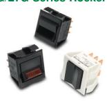
The TG-Series Mini Tippette rocker switches are single or double pole and feature an all nylon double-insulated construction. These switches are designed with snap-in mounting for fast, low cost assembly. The illuminated version (LTG) is available with either a paddle or rocker actuator. These AC rated switches are also suitable for low-voltage DC applications in a wide range of markets including Appliance, HVAC, Food service, and Transportation.
